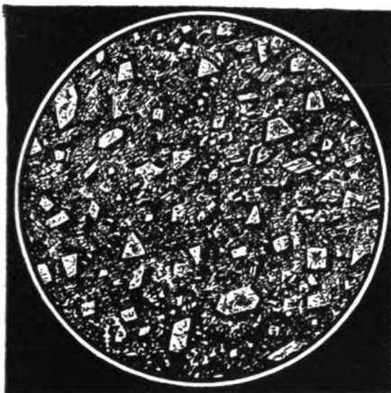
A magnified view of the structure of a fine grained anti-friction metal. The crystals and grains are soft
